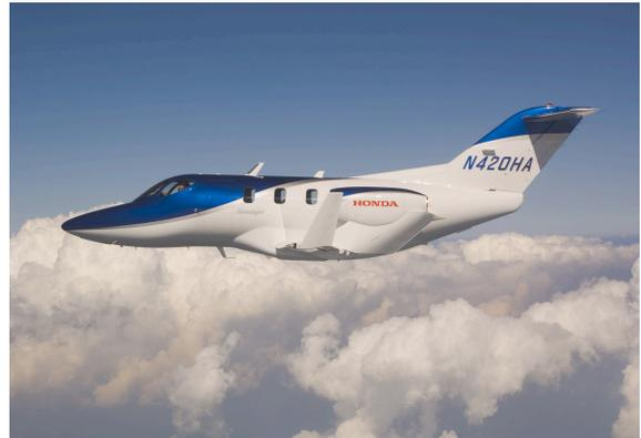
According to a company statement, the first production version of the HondaJet completed an 84 minute flight from its headquarters in Greensboro, N.C. During the flight, the aircraft climbed to 15,500 feet and reached 348 Knots True Airspeed (KTAS).
