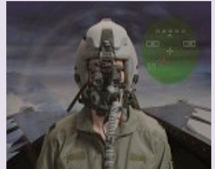
The DEP is a simple and cost-effective plug-and-play solution that enables pilots to transition from day to night configuration, improves situational awareness and meets the operational needs of military aviators. DEP can be installed onboard any fielded JHMCS, D-JHMCS or JHMCS-II.
