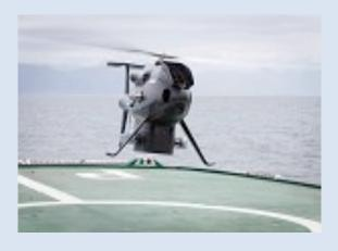
During the trials the payload of choice was the Selex ES SAGE Electronic Support Measure (ESM) system, rendering the CAMCOPTER® S-100 capable of detecting, identifying and geolocating radio frequency sources while it routinely operates out to ranges of 200 km or remains on-station for periods of more than 6 hours. This system provides the perfect support for maritime surveillance missions or anti-piracy operations in which the South African Navy was interested.
