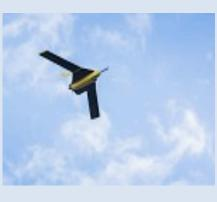
Fulmar, a small, high performance, fixed wing UAS, is to be installed on six New Generation Patrol Crafts (NGPC), being constructed by Destini Shipbuilding and Engineering Sdn. Bhd. The maritime design of Fulmar allows the aircraft to take-off and land, whilst the ship is in motion, a key requirement of the MMEA. This capability offers an unrivalled competitive advantage to other systems in the market.
